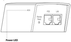
The Power LED indicates the status of the electric current: green (0~0.8A), red (0.8A~1A).
