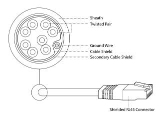
Shielded CAT5e (or above) Cable with Ground Wire
