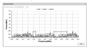
4. Close the Spectrum Analysis Window, and then you will get back to the 'WIRELESS' page. For the Channel/Frequency option, it is recommended to select a value whose frequency is within the noted frequency range.
