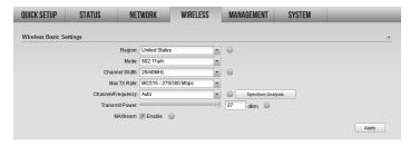
Pharos MAXtream is a non-standard Wi-Fi protocol that is only compatible with TP-LINK's Pharos series products. Please notice that you will not be able to connect other Wi-Fi devices to an AP with MAXtream enabled.
