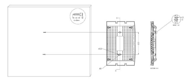
Figure 2-2 Wall-mount Installation
