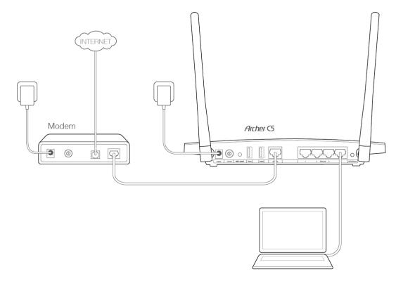
Figure 2-1 Hardware Installation
