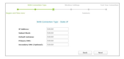
Figure 3-6 WAN Connection Type - Static IP
